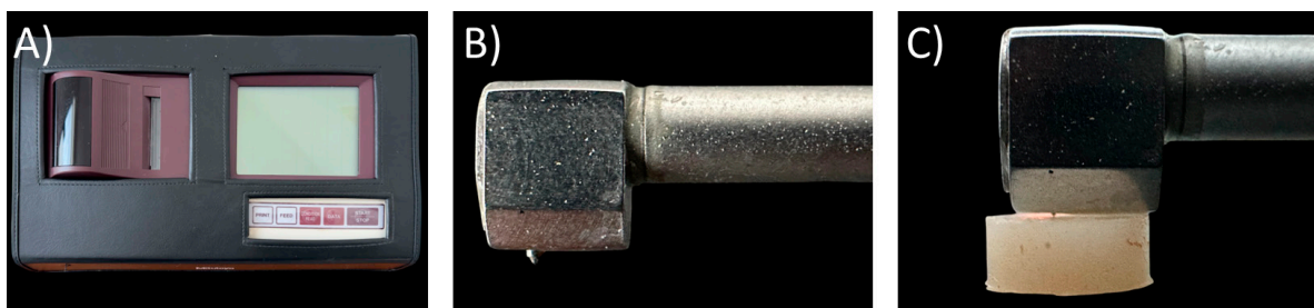
Figure 3. Roughness test. A. Roughness tester. B. Detector tip with a diamond stylus. C. Sample with detector tip.
