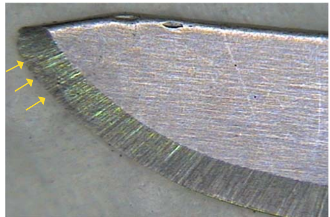
Figure 4. Elite® D3 scalpel blade after use. Edge opacity is noticeable in the sharp edge; this can be interpreted as physical deformation of the blade.
