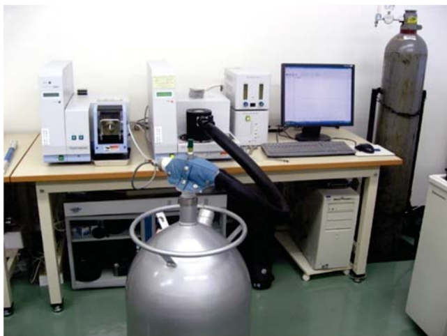
Figure 8. Nitrogen-based cooling system used in the test.
