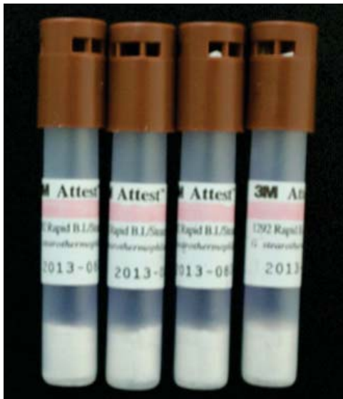
Figure 1. Rapid lecture biological indicators for autoclave use.
