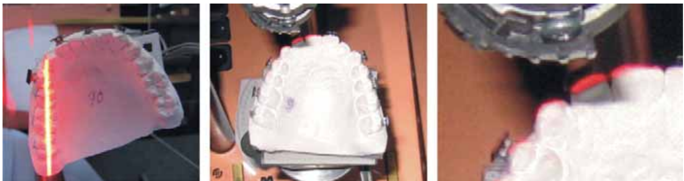
Figure 7. Laser beam guided over occlusal groove of posterior teeth and incisal borders.
