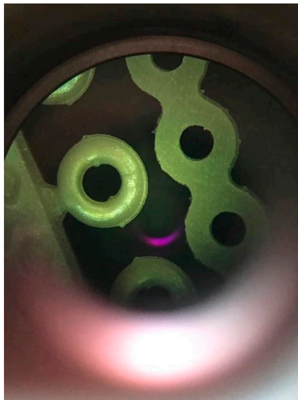
Figure 1. Optical microscopy image of 3M elastomeric module (injection) and 3M elastomeric chain (stamped).
