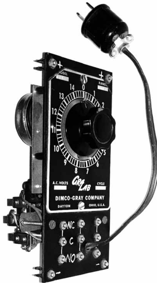
Figure 2. A Bakelite panel with a GraLab timer. The state of the contacts in an electromagnetic relay in the back of the panel changed when the timer was activated and deactivated. The coil in the relay and the motor of the timer worked with 110-120 V AC. Below the dial, a series of snap studs connected to the contacts of the relay, were used for connecting other devices using snap leads. The connectors in the upper and lower sections of the panel (marked + and -) were used for connection with rods in the relay rack.
