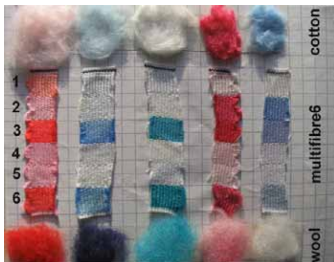
Figure 3. Pieces of multifiber 6, dyed with acid red 81, acid blue 25, acid green 50, direct red 81 and direct blue 1 (2 cotton, 3 nylon, 6 wool).
