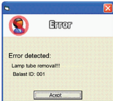
Figure 11. Fault condition window for lamp tube removal
