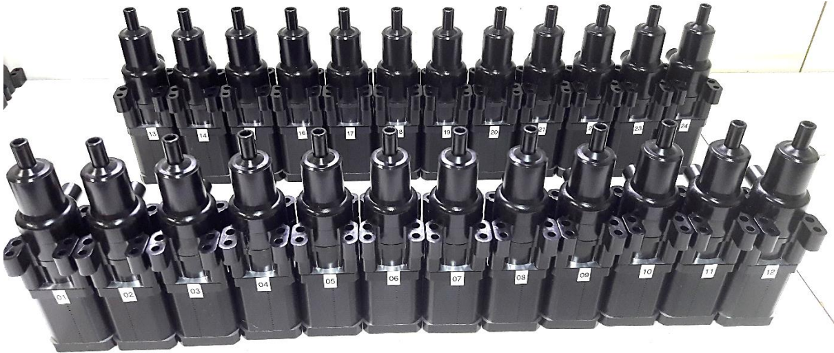
Figure 11. Image of the Percolore brand pumps assembled with its respective label indicated the test specimen (created by author).
