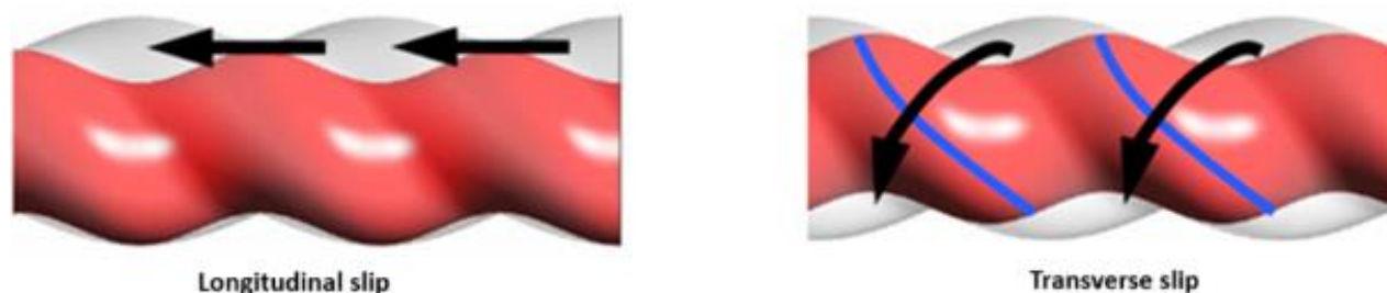
Figure 4. Representation of the slip mechanisms of a PCP (adapted from Paladino et al. , 2008).
