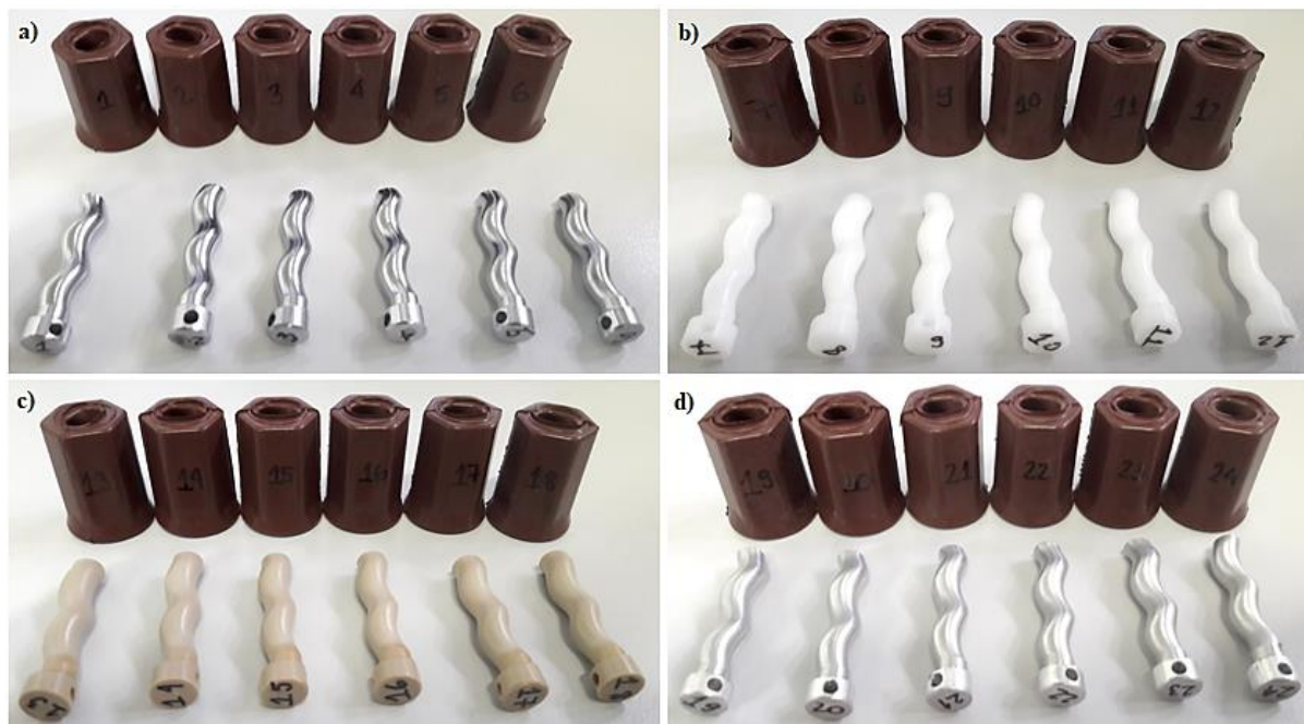
Figure 10. Rotors and their respective FKM stators. a) Chrome-plated SAE 12L14 steel rotors; b) PA6 rotors; c) PEEK rotors; d) 6082-T6 aluminum alloy rotors (created by author).
