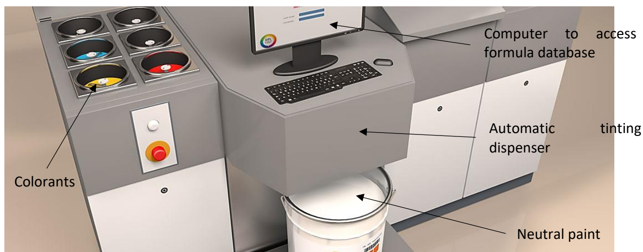
Figure 1. Main components of the automatic paint tinting dispensing system (Geltint, 2018).
