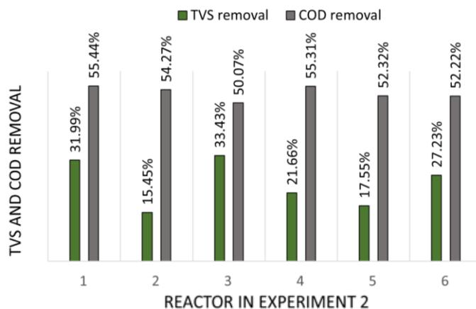
Figure 5. Variation of TVS and COD removal in Experiment II.
