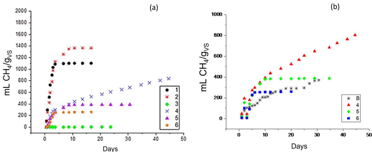
**Figure 6.** (a) Comparison of accumulated methane production under experimental conditions in Experiment II. (b) Comparison of accumulated production under experimental conditions with 50% vinasse and 50% elephant grass broth, from assays I and II, with and without addition of sodium bicarbonate. %V/C/A (alkalizer): 1 (50/0/50), 2 (75/0/25), 3 (0/50/50), 4 (50/50/0 - 0.05), 5 (50/50/0 - 0.11), 6 (50/50/0 - 0.25) e %V/C: B (50/50).
