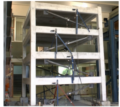
Figure 6: Héctor Guerrero Bobadilla, Reinforced concrete model tested on a shaking table at the UNAM. Image taken from: Héctor Guerrero Bobadilla, Seismic Design and Performance of Hospital Structures Equipped with Buckling-Restrained Braces in the Lakebed Zone of Mexico City . PHD Thesis Dissertation, University of Manchester, UK, 2016.
