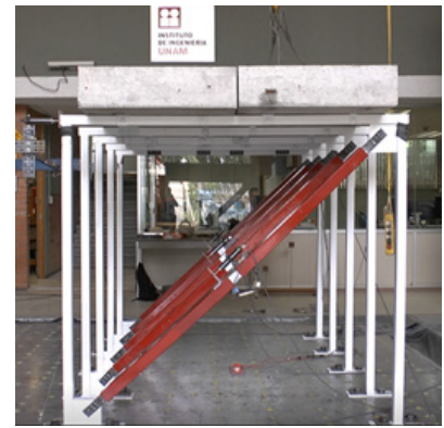
Figure 10: Héctor Guerrero Bobadilla, Five one-storey one-bay frames tested on a shaking table.
