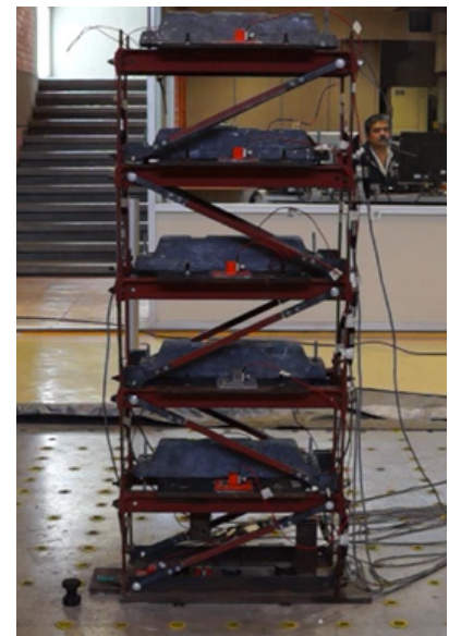
Figure 3: Héctor Guerrero, A Steel Frame Model Tested on a Shaking Table at UNAM. Image taken from: Héctor Guerrero Bobadilla and others, "Experimental studies of a steel frame model with and without buckling-restrained braces." Ingeniería Sísmica 95, (2017):33-52.
