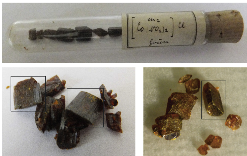
Figure 9 Top: The vial of Adolf Grün containing the [cis-dinitrobis(ethylenediamine)cobalt]Cl complex. Bottom left: The crystals of the vial of Adolf Grün. The crystals (see boxes) show a remarkable striation of the larger crystals indicating a layered growth process by twinning. Each striation stripe is supposed to correspond to a twinning layer. Bottom right: Edith Humphrey's crystals of [cis-dinitrobis(ethylenediamine)cobalt]Br do not show visible striation. The twinning layers of Edith Humphrey's bromide have apparently thicknesses below the visibility range.
