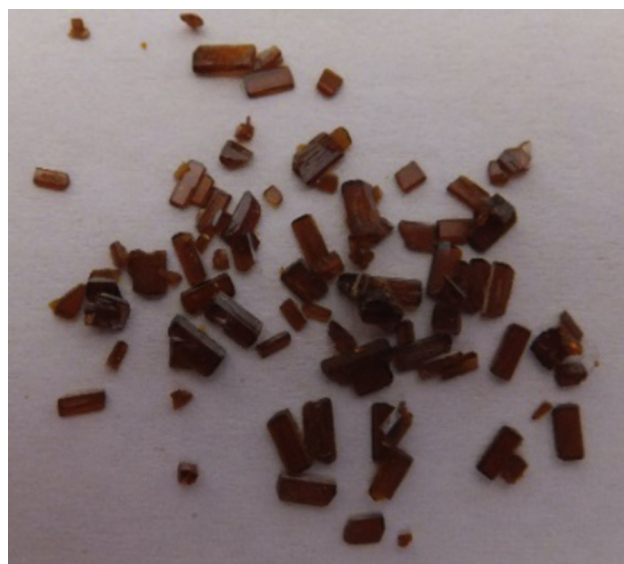
Figure 18 Crystals of [ \Lambda -dinitrobis(ethylenediamine)cobalt]Cl obtained by Richard Hessen via seeding of a saturated solution of the racemic [dinitrobis(ethylenediamine)cobalt]Cl complex with crystals of the [ \Lambda -dinitrobis(ethylenediamine)cobalt] chloride.
